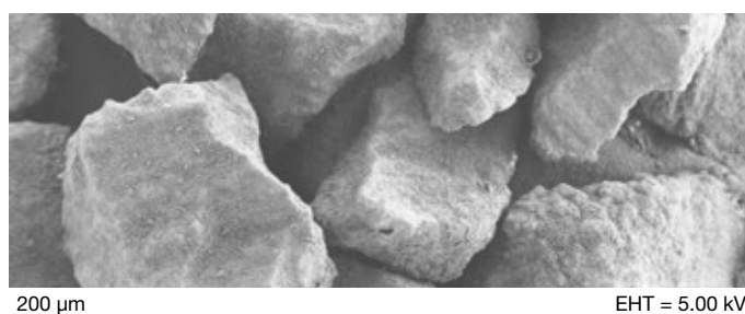
Figure 1. Scanning electron microscopy (SEM) image of cetirizine HCl (SE, 5 kV).
